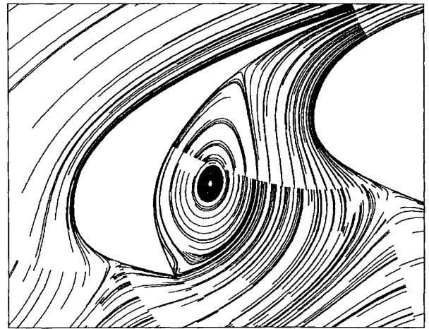
Fig. 12 Streamlines on the lower surface of the slat for the GA(W)-1 airfoil with slat and flap.
